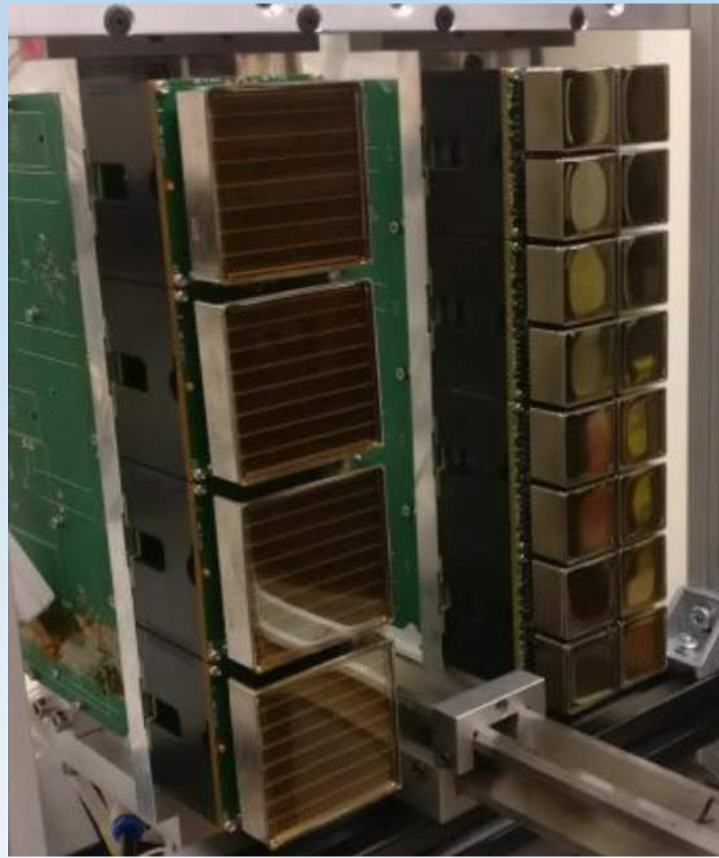
Quality control for 3,600 MaPMTs for LHCb upgrade
